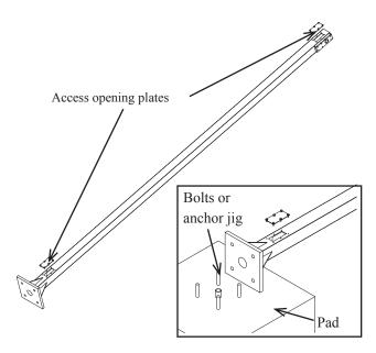
Figure 5 Placement of Pole on Pad
